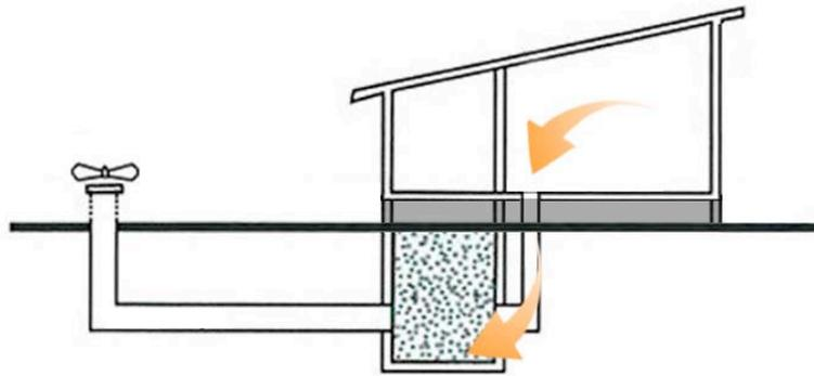
Fig. 7b *Direct Ground Cooling – Earth as a heat sink* (adapted from Koch-Nielsen H. 2002, p135)
